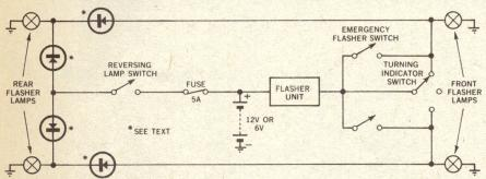
The addition of four diodes, a reversing light switch, and a fuse, added to a conventional flasher circuit, enables the flasher lights to double as reversing lights.
